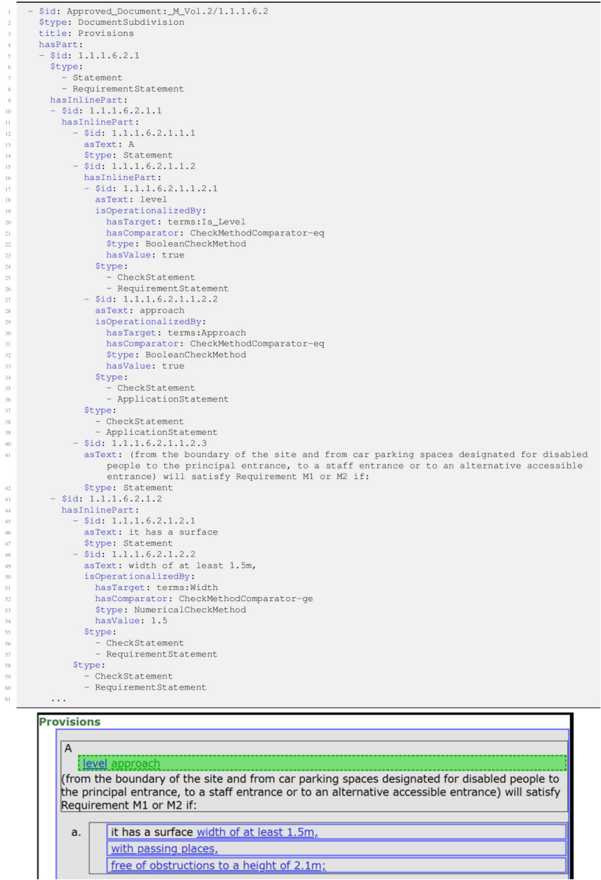
Figure 17.10 RASE annotations and corresponding metadata in BCRL (YAML) format. The corresponding annotations are graphically illustrated in the diagram below.
