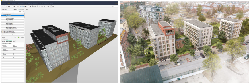
Figure 18.3 The structural view of an IFC model in the Solibri software (left side) and the same IFC model used as visualisation material, combined with city model views that display the actual buildings and the surrounding environment (right side).
