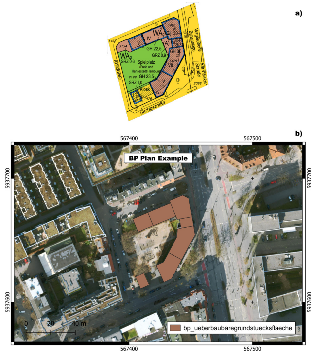
Figure 12.2 (a) BPlan test data and (b) 2D spatial data representing the BP_UeberbaubareGrundstuecksFlaeche class.
