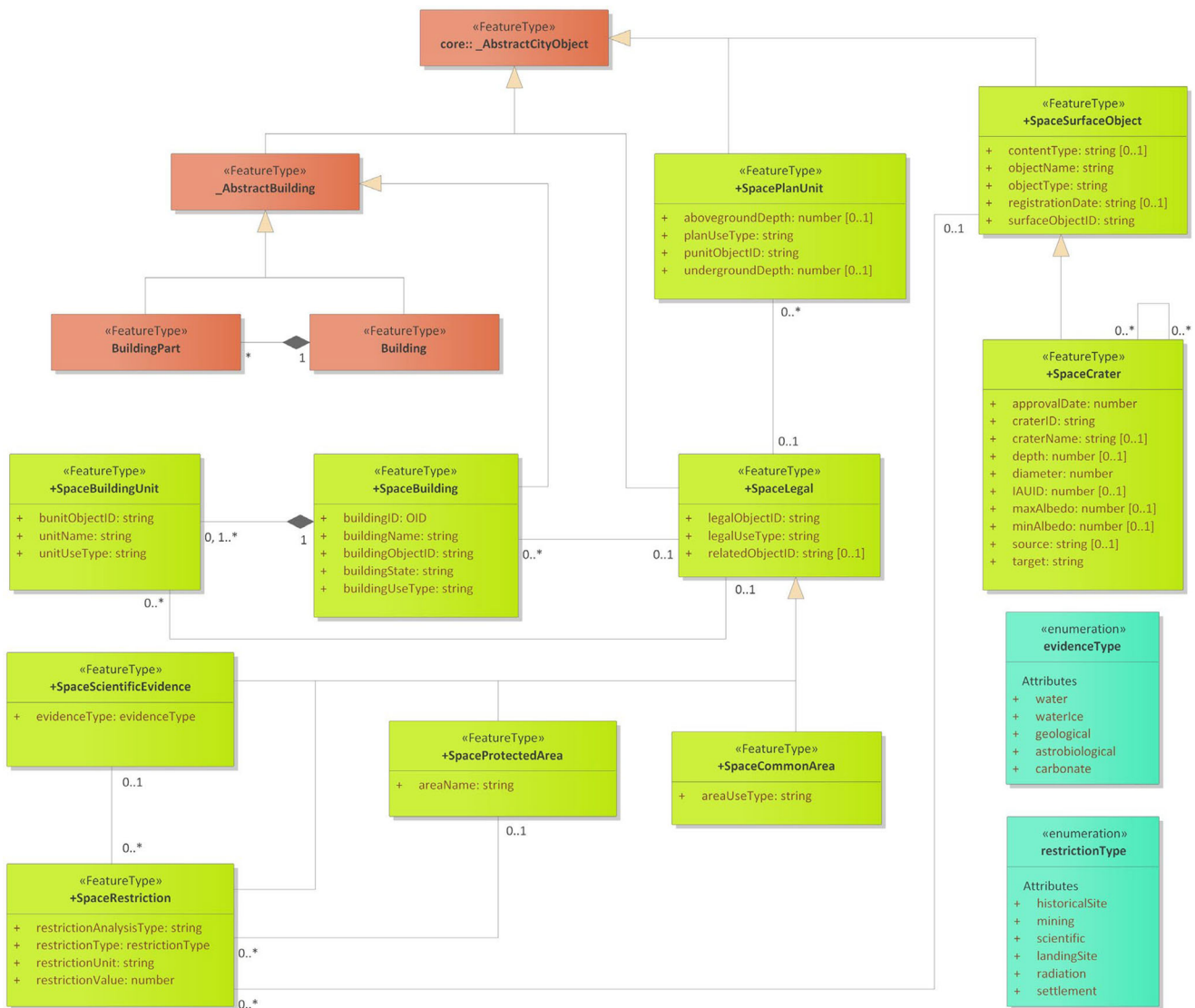
Fig. 2 The conceptual model of the developed standard extension that enables 3D modeling of different types of surface/subsurface objects and related logical spaces on celestial bodies
