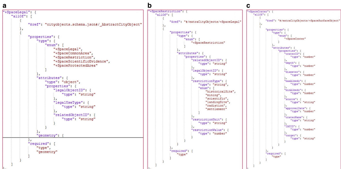
Fig. 3 The selected parts of the created CityJSON extension file
